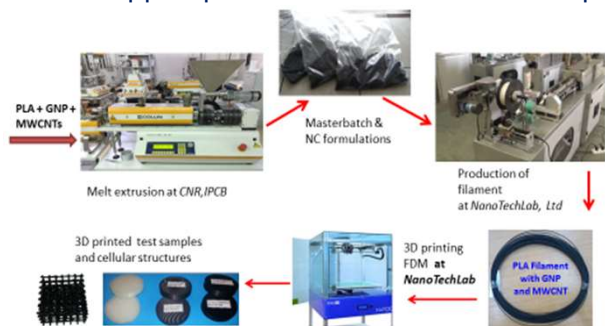
Fig.1. Production line for PLA based nanocomposite filament
